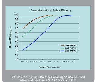
The Camfil Farr Durafil® 2V provides high-efficiency performance in a compact, energy-efficient design. The Durafil 2V:
